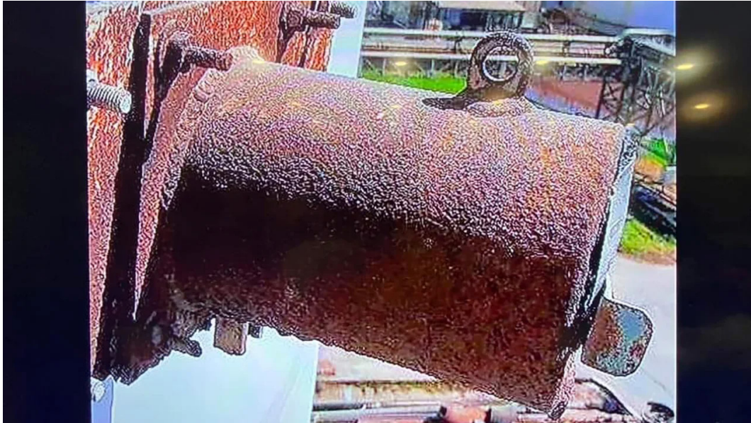
This image, provided by the Prachinburi Provincial Public Relations Office, shows the missing radioactive cylinder as part of a steel tube.
