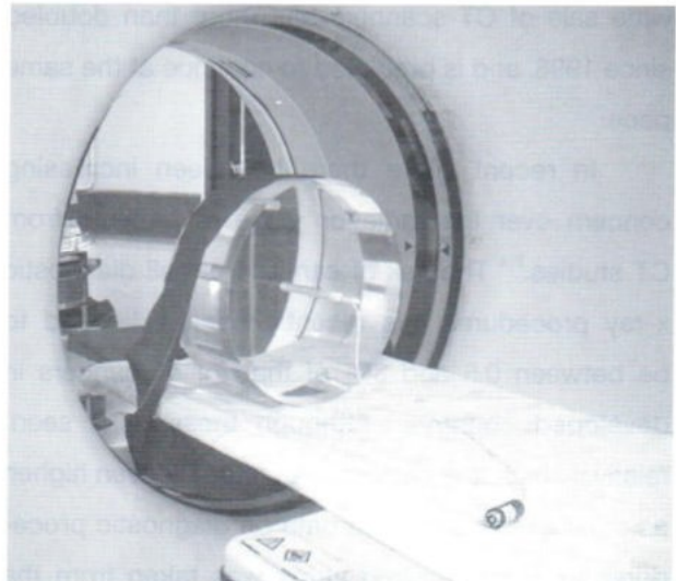
Fig.3 Body CT Phantom diameter 32 cm with 100 mm pencil ion chamber set at the center of the gantry for CTDI measurements.
