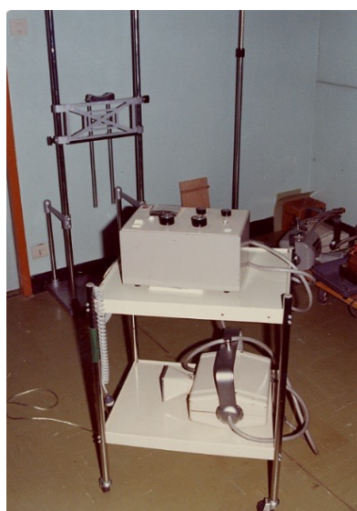
Figure 10. X-ray control device; tube voltage was 100kV; tube current was 20mA, and the exposure time was 0.1 to 10 seconds.
