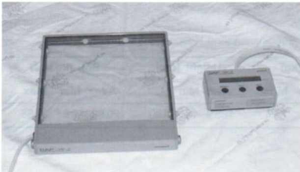
Fig.3 DAP detector and Meter PTW Model Pehamed W 2
