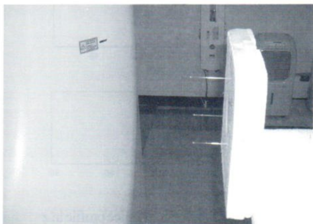
Fig.1 Capillary point sources were suspended by a fixture.
