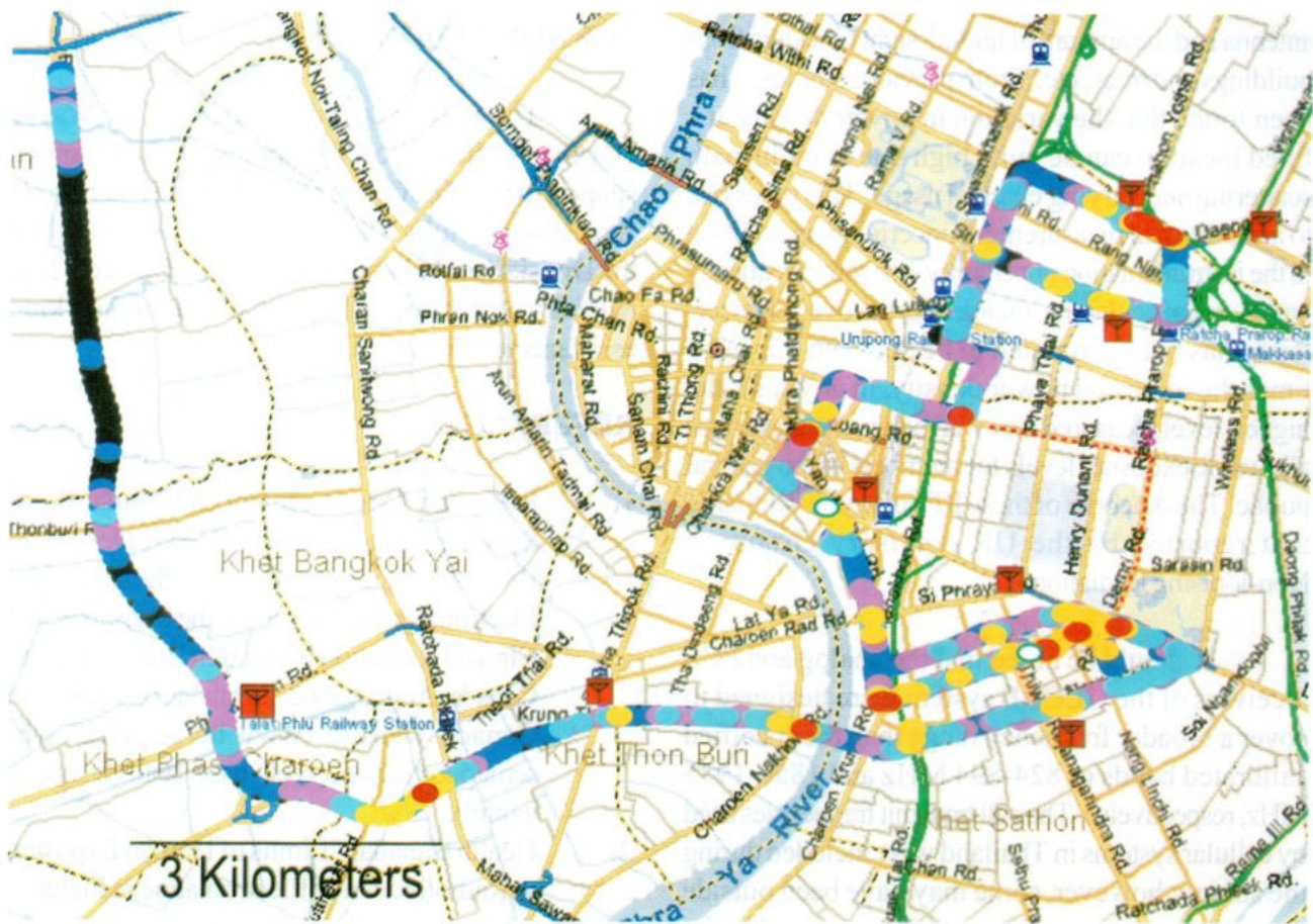
Fig.4 PCS-band power density map of outer and inner Bangkok (Ratchapluak, Krung Thon Buri, South Sathon, North Sathon, Rama IV, Silom, Surawong and Si Phraya Roads)
