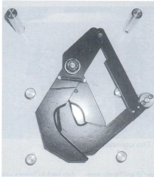
**Fig.3** Metal jaws to simulate the beating heart
