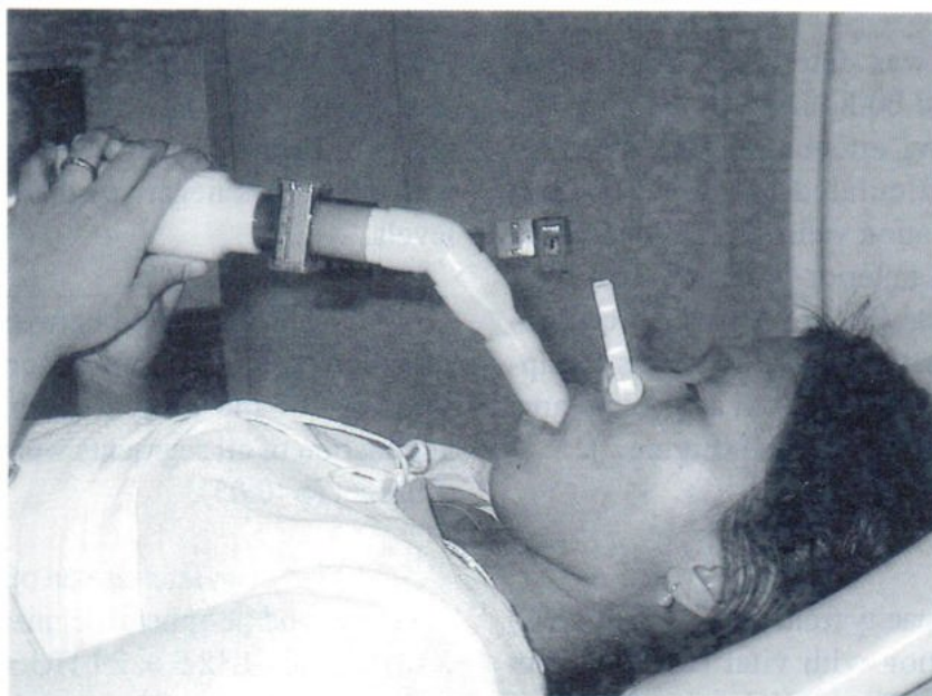
Fig. 2. The spirometer gating device with application in a volunteer study.
