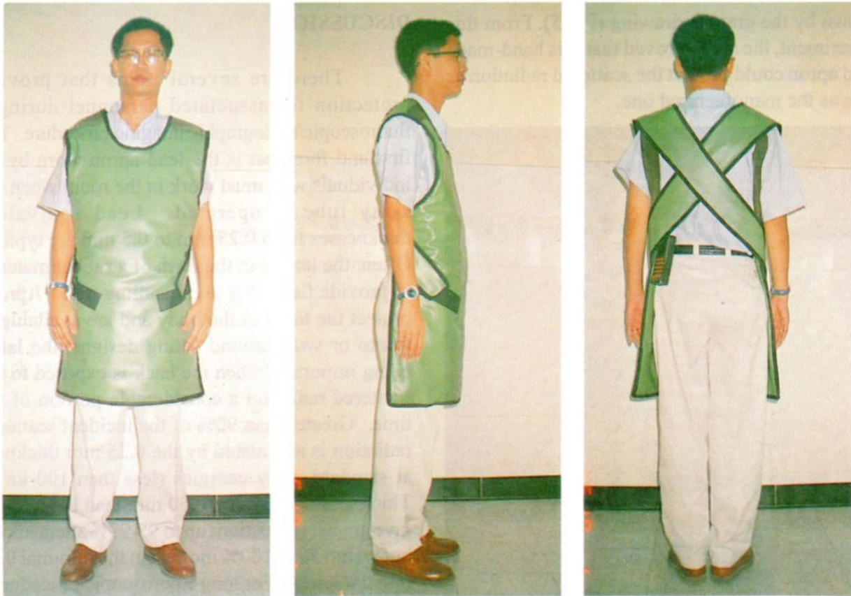
Fig. 4 The hand-made body lead apron on the real technician.
