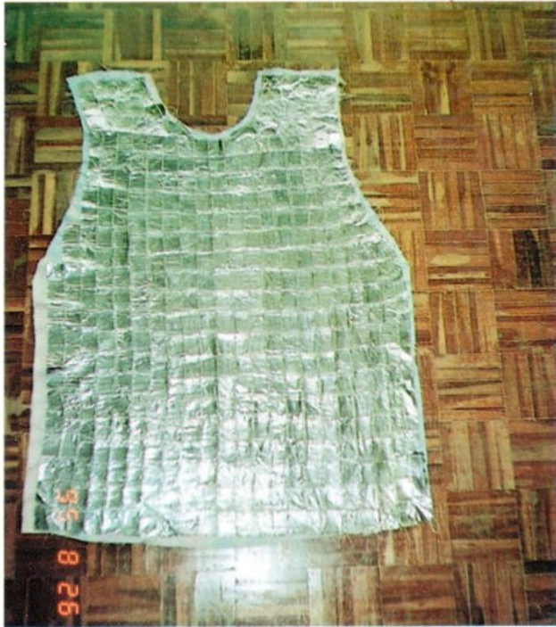
Fig. 2 Lead sheets sewed on the thin piece of cloth
